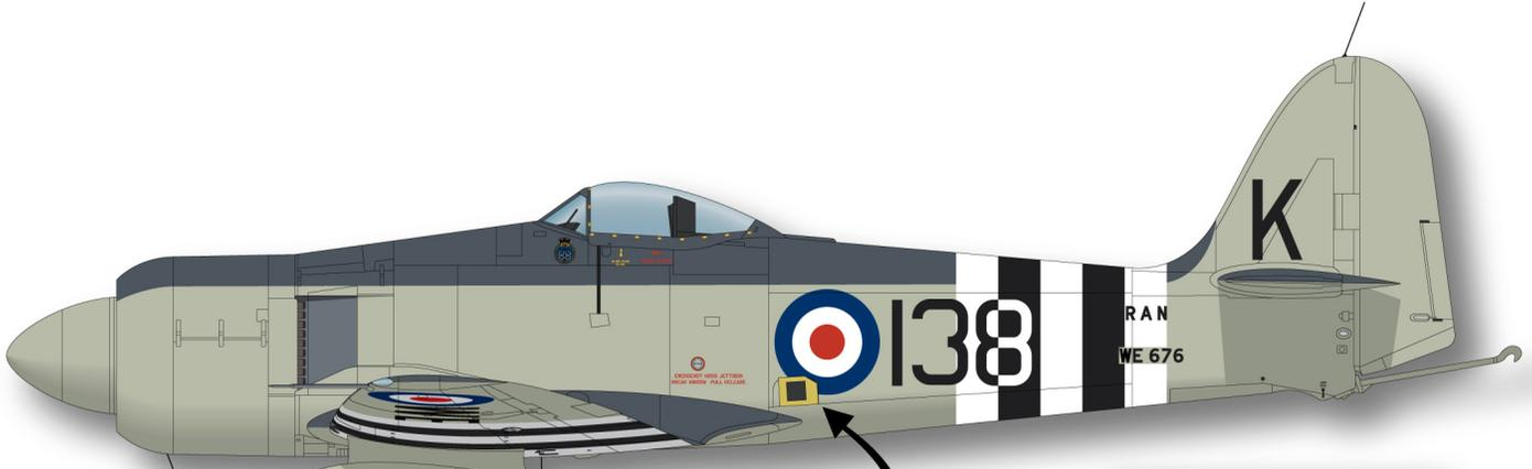
WE676 was fitted with an oblique camera port. It appears that the sheet metal around the camera window was painted yellow zinc chromate.
