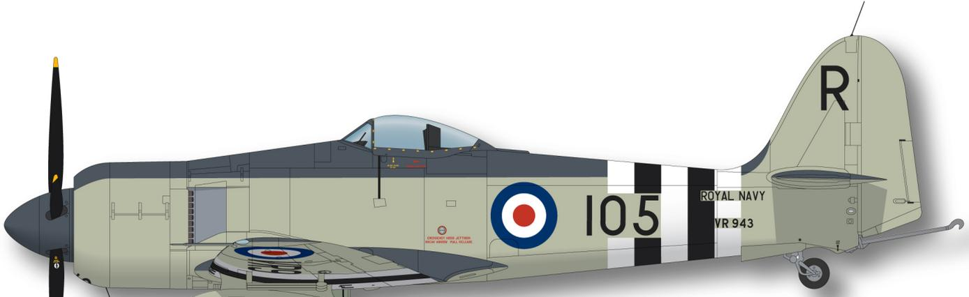
Number is oriented parallel with ground line when aircraft is standing on its gear.
