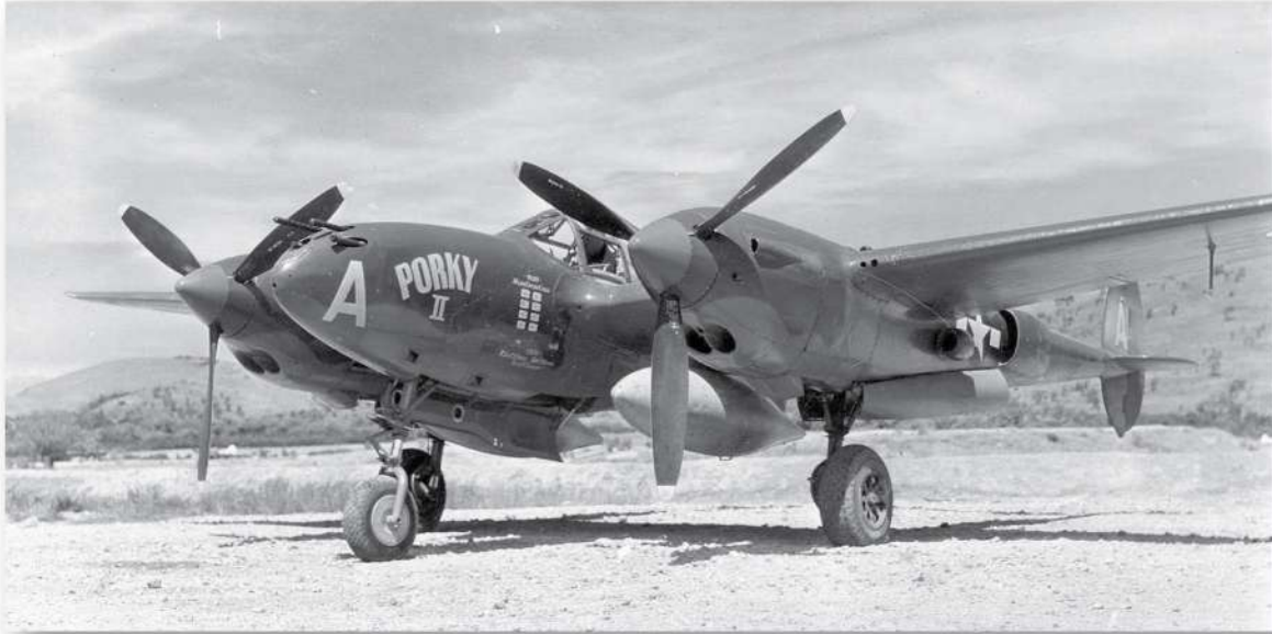
"Porky II" showing her covered nose, and uncovered main wheel hubs. Again, note the light grey Mk.6 tanks - noticeably lighter than the Neutral Gray belly of the aircraft. Cragg's ship appears to be fairly well maintained (given the conditions...). Note the ubiquitous light brownish grey exhaust and tetraethyl lead stains on the boom and the vertical fin.
