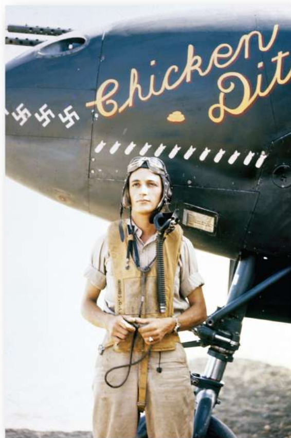
A youthful looking Gerald Rounds poses in front of his P-38G "Chicken Dit". Note the tape over the shell ejection chute - dust was an ever-present enemy in the Mediterranean and North Africa.
