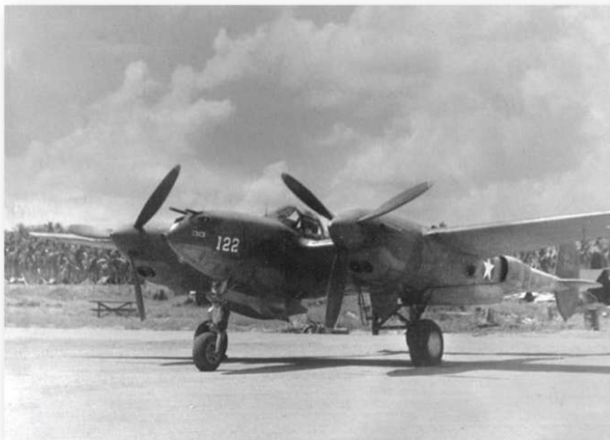
Two photos showing Lanphier's rather plainly marked "Phoebe". Note that the "122s" on the nose were applied at an angle to the longitudinal axis of the aircraft. Also note her uncovered nose wheel hub and covered mains. Otherwise she was a very bog standard looking P-38G.
