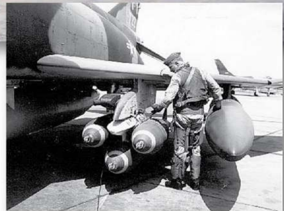
A trio of Mk.117 750 lb iron bombs loaded on a TER under the inboard pylon. Note that during the time period covered here, the AIM-9 launch rails could not be fitted when other ordnance was loaded on the inboard pylons.
