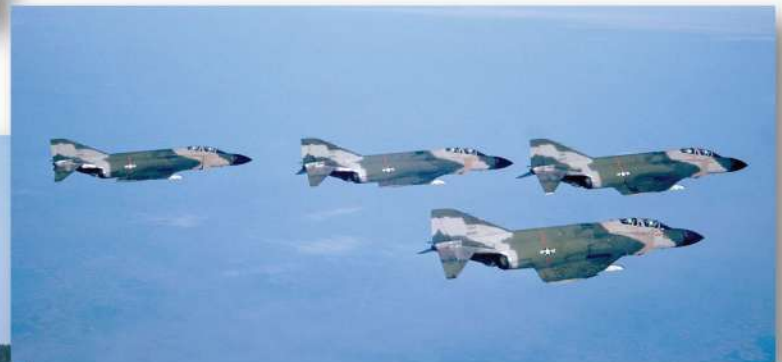
Some examples of the McDonnell factory applied camouflage seen on 64-0927. Both the colors and the pattern used by McAir were non-standard. Also note the borderless national insignias on the fuselage (and upper wing), the full turbine warning stripe, and the Futura font style warning placards around the nose. The belly was in the correct FS 36622 on these aircraft.
