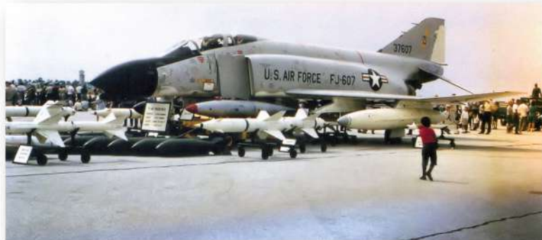
F-4C-20-MC 63-7607 showing the Air Force standard markings of this period. Note the addition of a red and white weapons loading placard, and the retention of the Navy style inboard pylon, plus McDonnell 370-gallon wing tanks with Corroguard trim. This aircraft was converted into an EF-4C Wild Weasel, and survived the ordeal in SEA, retiring to AMARG in 1991.
