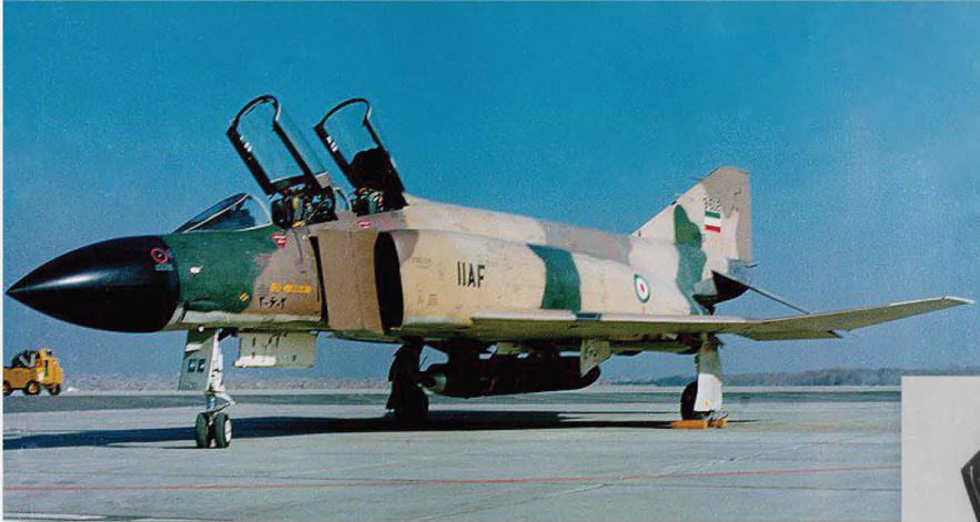
Right: IIAF Commander-in-Chief Gen. Khatami climbs aboard F-4D-37-MC 68-6910 (3-623), delivered 7 Jul 69. Absolutely standard factory 'Asia Minor' camouflage and stencils. Note the very visible internal canopy fiberglass sealing strips.
