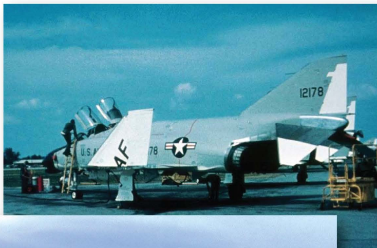
A great early shot of RF-4C-27-MC, 65-0903 showing the factory applied gloss black on the inboard halves of the stabilizers and the translating ring on the afterburner nozzle.
