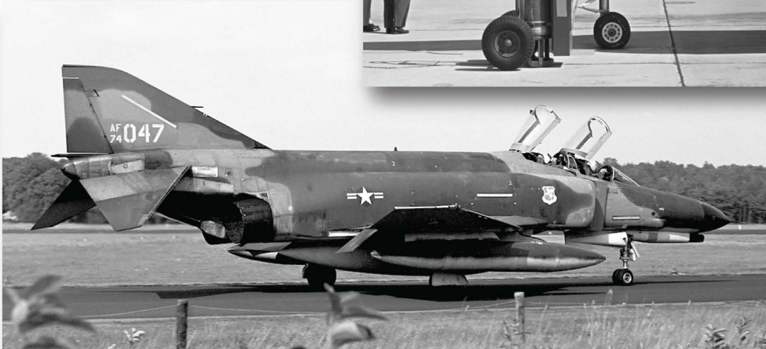
Below: a late production F-4E-60-MC wearing her full factory camouflage and markings. She has some white dots, but is not covered with them as was seen on many aircraft. We can't explain the difference.
