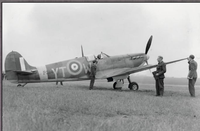
No. 65 Squadron Spitfire Mk.IIa, P8147, at RAF Kirton in Lindsey in the summer of 1941. This aircraft is equipped with a De Havilland 5/39A constant speed propeller. Note the atypical bottom surface painting and fuselage band. Metal ailerons are possible on this aircraft. (photo: Simon Erland)
