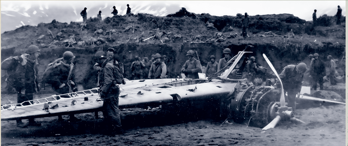
American soldiers in May 1943 at the wreck of the Rufe in Holtz Bay on Attu Island. Part of the oil cooling system is visible on the main pylon structure.
