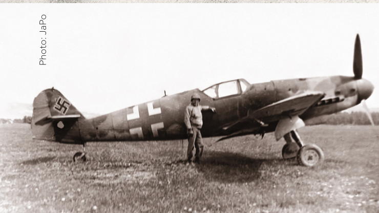
A late war production Bf 109 K-4 probably with RLM 81 (dark brown) and RLM 82 on fuselage on a photo from Salzburg, Austria at the end of war. Yellow markings on rudder and engine cowling were introduced by Luftflotte 4 in March 1945.
